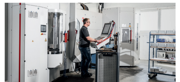
top The Hermle manufacturing cell at HZT Honermeier, consisting of the C 400 U 5-axis machining centre and the HS flex automation solution.
