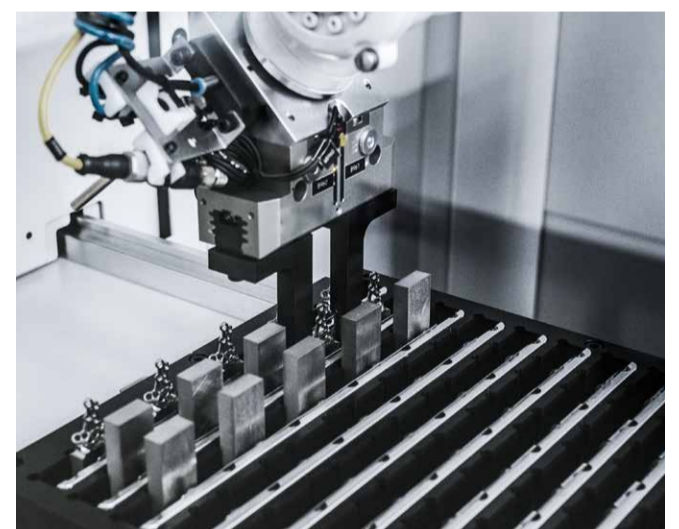
A workpiece pallet designed by Medartis with multiple holding fixtures for supplying titanium blanks or holding finished parts with fully automated robot handling.
