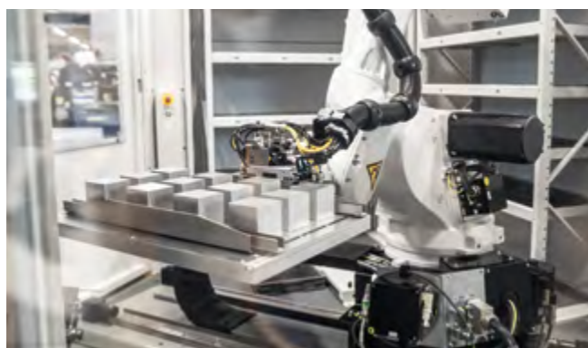
above The universal die adapts flexibly to various geometries.
