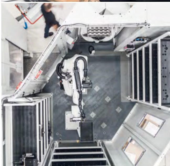
top The SOFLEX software facilitates operation - of both the 5-axis machines and the adapted automation. bottom The C 400 U is automated with the RS 1 robot system - perfect for parts handling when machining standard products.
