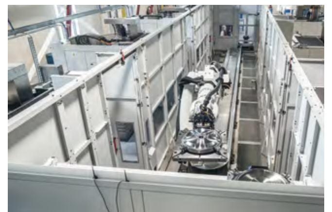
above The robot reaches each of the six C 42 V machining centres via a linear axis.
